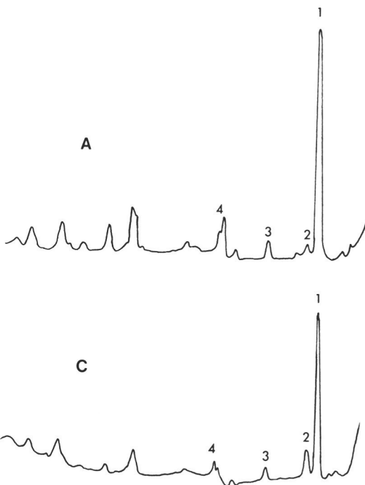
Fig. 2 —Solid-sample gas chromatograms of the head of one Atta cephalotes media worker, on a 5 % Carbowax column. Trace reads from right to left; temperature program : 4° per min increase from 70° to 190°C. A and C indicate the colony of origin. 1 is 4-methyl-3-heptanone, 2 is 2-heptanone, 3 and 4 are probably 3-octanone and 3-octanol respectively.
